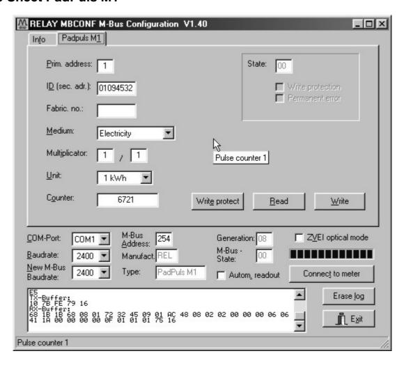
These sheet shows the actual settings and values of the PadPuls M1. The following input boxes and buttons are used to change the params of the pulse adapter:
