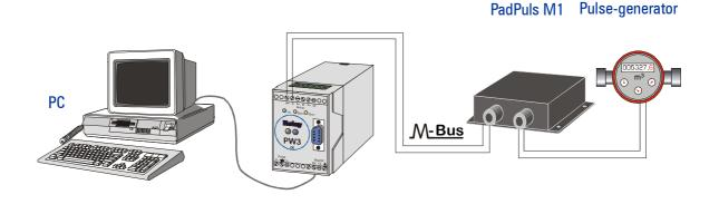
After opening the housing please lead the M-Bus cable through the left cable gland of the cover and connect the cable to the left terminal. Then do the same with the cable of the pulse generator (right side). Please connect an optional shielding to the terminal labeled with "Schirm". Connect the shielding only at the PadPuls.
