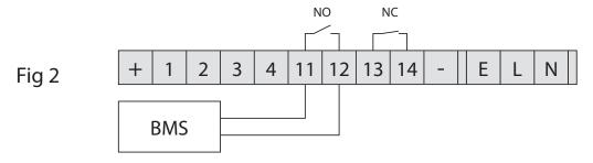
Connection to Building Management System - BMS Normally open contact closes in Alarm situation
