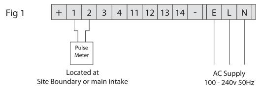
Connection of electric supply and pulse water meter
