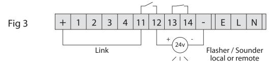
Connection of 24v DC Flasher / Sounder - activated in Alarm situation
