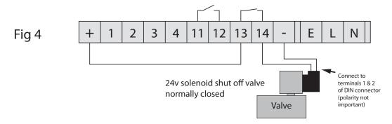
Shut off valve - valve is normally energised via NC contact allowing water to flow. In alarm situation valve closes - shutting off water.
